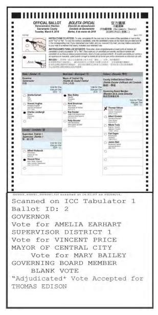
mark. The pixel count of each mark is compared with two thresholds (which are customer configurable, to determine what constitutes a vote.
